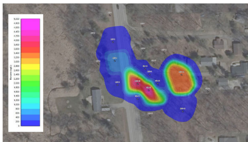
Figure 1. Six Months Pre-Injection, Benzene in Groundwater Concentrations
